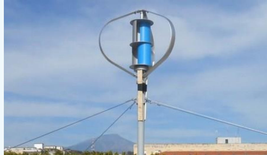
300W turbine installed for educational didactic purposes at the Archimedes Technical Institute of Catania
